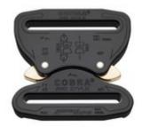
The COBRA® PRO STYLE is the world leading safety buckle made of aluminium. Thanks to its patented locking mechanism and high breaking strength it meets the highest safety requirements. In combination with a fitting webbing, the minimum guaranteed load capacity is 9 kN tensile strength and 18 kN in loop configuration.
