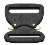
The COBRA® PRO STYLE is the world leading safety buckle made of aluminium. Thanks to its patented locking mechanism and high breaking strength it meets the highest safety requirements. In combination with a fitting webbing, the minimum guaranteed load capacity is 9 kN tensile strength and 18 kN in loop configuration.
