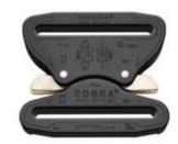
The COBRA® PRO STYLE is the world leading safety buckle made of aluminium. Thanks to its patented locking mechanism and high breaking strength it meets the highest safety requirements. In combination with a fitting webbing, the minimum guaranteed load capacity is 9 kN tensile strength and 18 kN in loop configuration.
