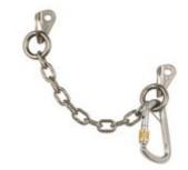
Belay station with two 10 mm bolt hangers, a chain, and a D-shape carabiner with screwlock and splint. The recommended drill hole distance needs to be 25-30 cm.
